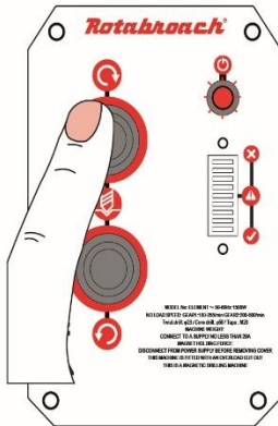
3) Motor OFF Press the top button on the control panel again. Once pressed the green illumination will no longer light up, this means the motor has stopped.
