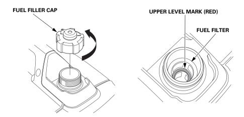
After refueling, tighten the fuel filler cap securely.
