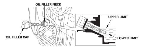
The Oil Alert system will automatically stop the engine before the oil level falls below safe limits. However, to avoid the inconvenience of an unexpected shutdown, check the oil level regularly.
