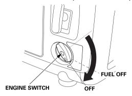
Operating the generator in the FUEL OFF position before turning the engine switch to the OFF position can reduce the fuel in the carburetor.
