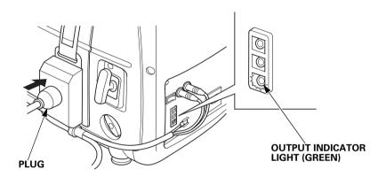
If the generators are overloaded (see page 36), or if there is a short circuit in a connected appliance, the overload indicator (red) will go ON. The overload indicator (red) will stay ON, and after about four seconds, current to the connected appliance(s) will shut off, and the output indicator (green) will go OFF. Stop both engines and investigate the problem.
